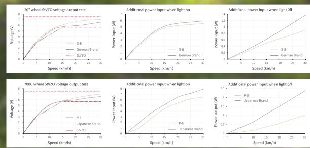
S-8 Series dynamo hubs are not only the smallest in its appearance, but also are the lightest at the market. This model is designed for wheel size from 400 to 536mm at a 6V3W rating. It is also ready for use with 700C wheels at 6V2.4W output. Meet small and light.
